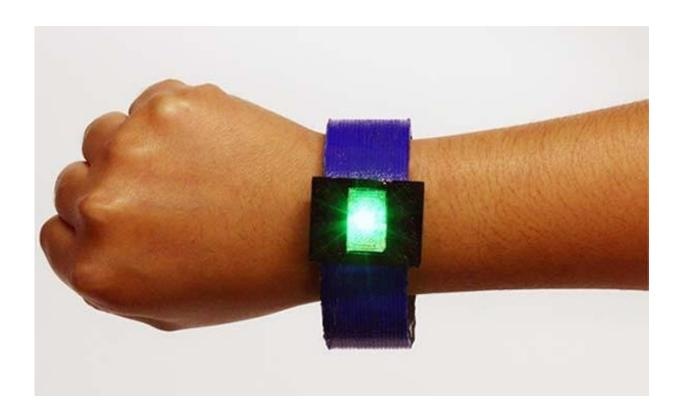
LED bangle, including a lithium-ion battery, was made entirely by 3D printing. Credit: American Chemical Society
