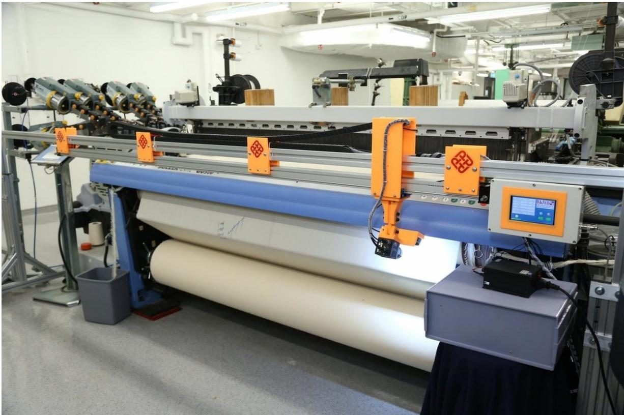
"WiseEye" has been put on trial for over six months in a real-life manufacturing environment. Results show that the system is able to reduce 90 percent of the loss and wastage in fabric manufacturing process. Credit: The Hong Kong Polytechnic University
