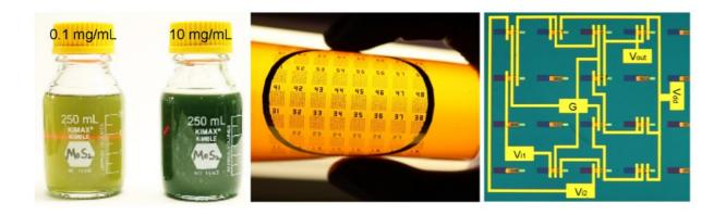
Solution-processable large-area electronics from MoS2 2D nanosheets ink. Credit: Duan Lab @UCLA Department of Chemistry & Biochemistry
