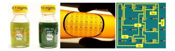
Solution-processable large-area electronics from MoS2 2D nanosheets ink. Credit: Duan Lab @UCLA Department of Chemistry & Biochemistry
