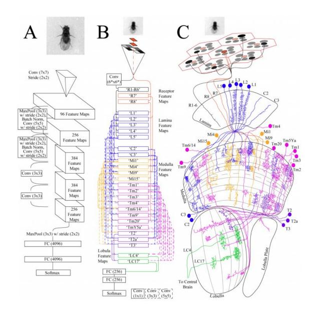
A) Modern Deep Convolutional Network machine learning algorithm B) Machine learning algorithm based on fly biology C) Connections in the fruit fly visual system. Credit: Schneider et al
