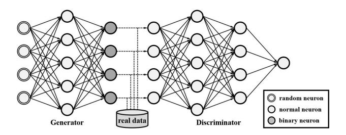
System diagram of the proposed model implemented by MLPs. Note that binary neurons are only used at the output layer of the generator. Credit: Dong and Yang.
