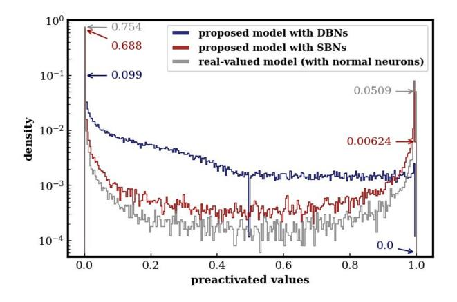
Histograms of the preactivated outputs for the proposed model and the probabilistic predictions for the real-valued model. The two models are both implemented by MLPs and trained with the WGAN-GP objective. Credit: Dong and Yang.
