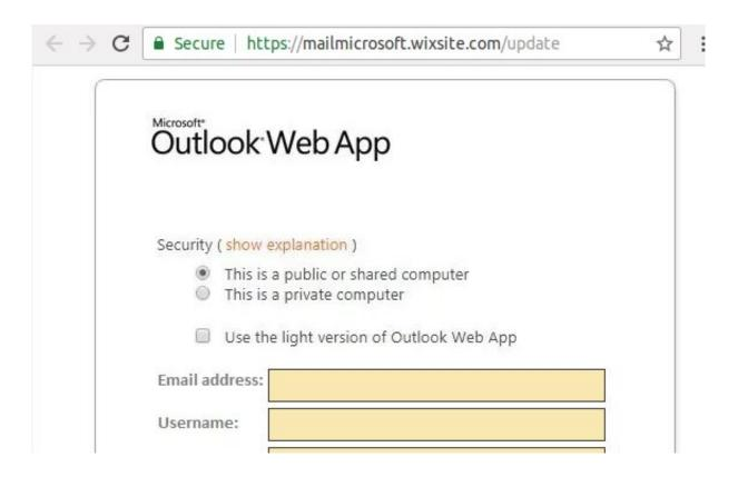
Example of phishing attacks using TLS. Credit: Torroledo, Camacho & Bahnsen
