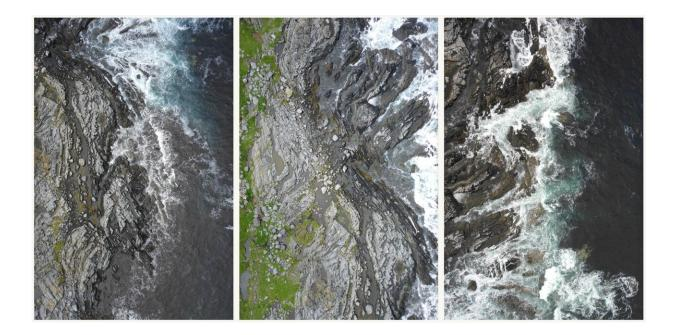
When the drone flies 100 meters above the ground, it takes pictures with a 3 x 3 cm resolution. This is 1,000 times better than a satellite, which takes pictures with a 30 x 30 m resolution. Credit: NIVA
