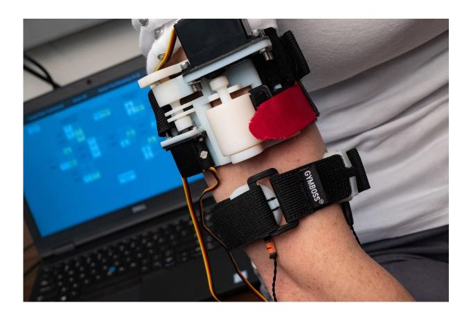
A new study by researchers from Rice University's Mechatronics and Haptic Interfaces Laboratory found users needed less than two hours of training to learn to "feel" most words that were transmitted by a haptic armband that communicates with signals comprised of squeeze, stretch and vibration. Credit: Jeff Fitlow/Rice University
