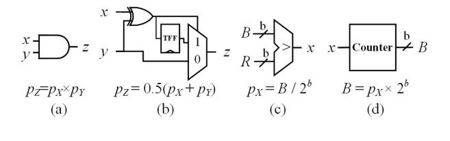
An example of stochastic computing circuits. SC circuits: (a) multiplier, (b), scaled adder, (c) digital-to-stochastic converter, and (d) stochastic-to-digital converter. Credit: Lee et al.
