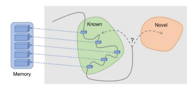
How the method works: observations are added to memory, reward is computed based on how far our current observation is from the most similar observation in memory. The agent receives more reward for seeing observations which are not represented in memory yet. Credit: Savinov et al.
