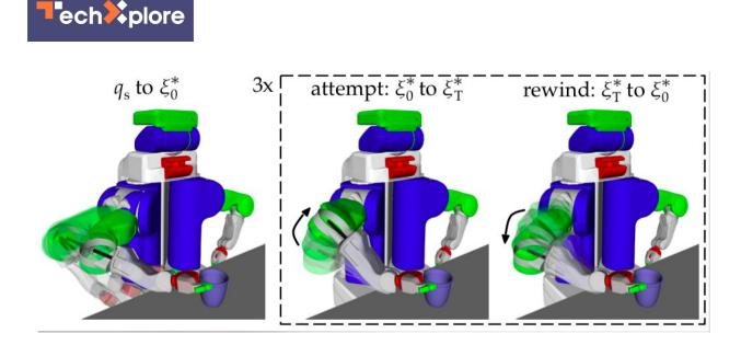
For a given incompletable task, the robot first executes the task until the point of failure (left), at which point it executes the attempt trajectory  $\xi *$  (center). To emphasize this motion, the robot then executes the reverse of  $\xi *$  to rewind back to  $\xi * 0$  (right), and repeats this two more times. Credit: Kwon, Huang and Dragan.
