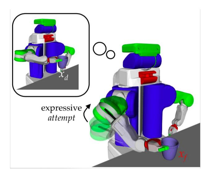
The method devised by the researchers generates an attempt motion meant to resemble successful execution (e.g., moving the end-effector from xf to xd) while obeying the constraints on the robot's limitations. In this example, lifts its elbow to communicate that it is trying to lift the cup, but the cup is too heavy to be lifted by it. Credit: Kwon, Huang and Dragan.
