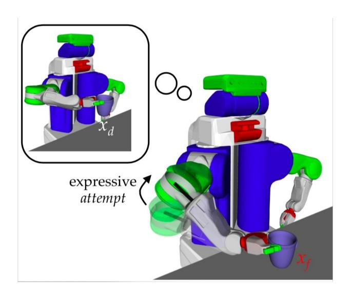
The method devised by the researchers generates an attempt motion meant to resemble successful execution (e.g., moving the end-effector from xf to xd) while obeying the constraints on the robot's limitations. In this example, lifts its elbow to communicate that it is trying to lift the cup, but the cup is too heavy to be lifted by it. Credit: Kwon, Huang and Dragan.
