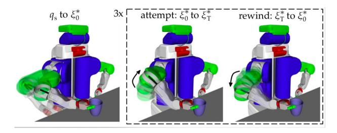
For a given incompletable task, the robot first executes the task until the point of failure (left), at which point it executes the attempt trajectory  $\xi$  \* (center). To emphasize this motion, the robot then executes the reverse of  $\xi$  \* to rewind back to  $\xi$  \* 0 (right), and repeats this two more times. Credit: Kwon, Huang and Dragan.
