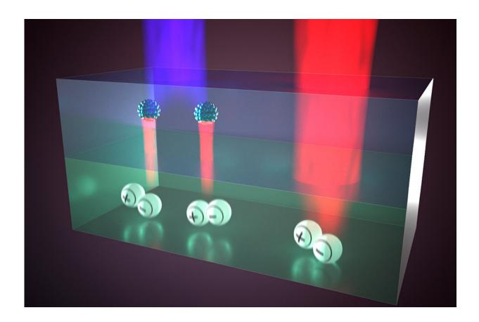
The singlet fission photon multiplier converts high energy photons into two low energy photons, which can efficiently be transformed into electric energy by the solar cell. Without singlet fission, the high-energy light would lose a large part of its energy to heat. Credit: Henk-Jan Boluijt
