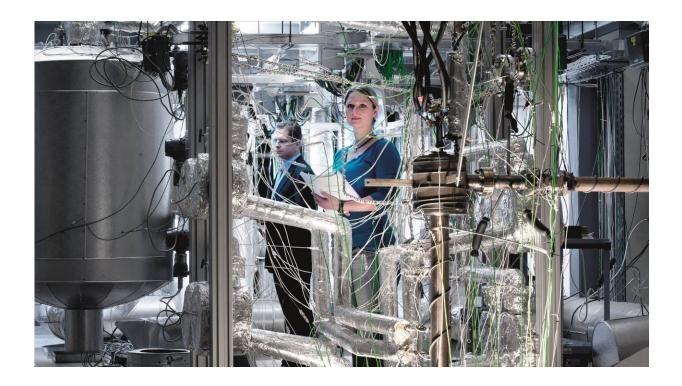
Test facility for liquid metals at KIT. Liquid metals are particularly suited for transferring high heat outputs. One of the objectives of NADINE is to study their use in thermal energy storage systems. Credit: Karsten Litfin/KIT
