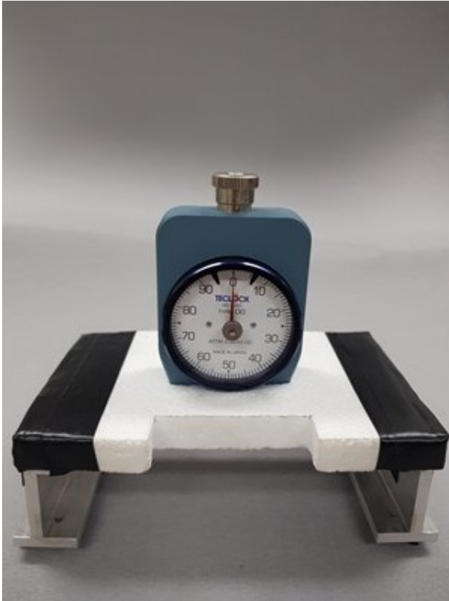
Figure 2. The instrument used for measuring human thermal status through skin hardness. Credit: The Korea Advanced Institute of Science and Technology (KAIST)
