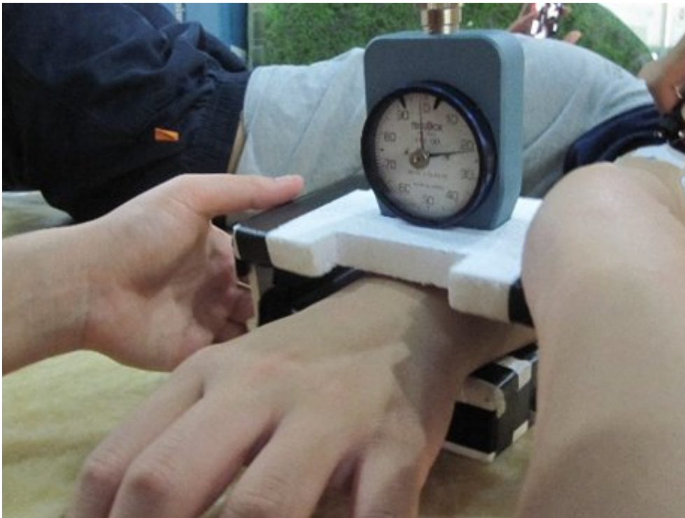
Figure 1. Measuring human thermal status through skin hardness. Credit: The Korea Advanced Institute of Science and Technology (KAIST)
