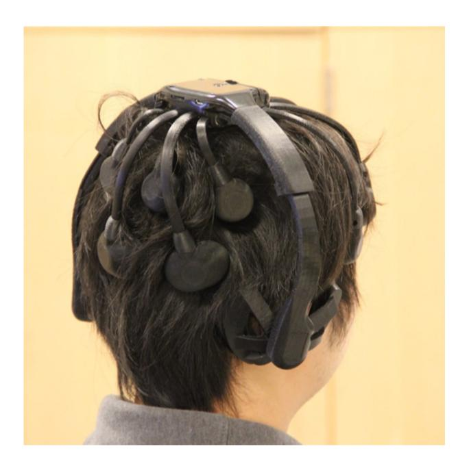
Three electrodes high on the back of a user's head are enough to detect a brain password. Credit: Wenyao Xu et al., <a href="CC BY-ND">CC BY-ND</a>
