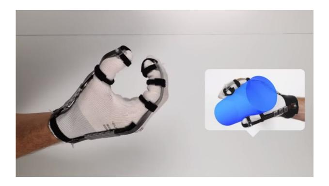
Scientists from EPFL and ETH Zurich have developed an ultra-light glove – weighing less than 8 grams per finger– that enables users to feel and manipulate virtual objects. Their system provides extremely realistic haptic feedback and could run on a battery, allowing for unparalleled freedom of movement.
