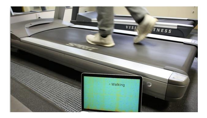
Carnegie Mellon University researchers are using laser vibrometry -- a method similar to one once used by the KGB for eavesdropping -- to monitor vibrations and movements of objects, enabling smart devices to be aware of human activity. Credit: Carnegie Mellon University
