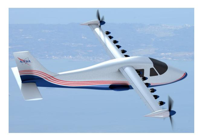
This artist's concept of NASA's experimental electric plane design shows 14 motors along the wings. Credit: <u>NASA</u>
