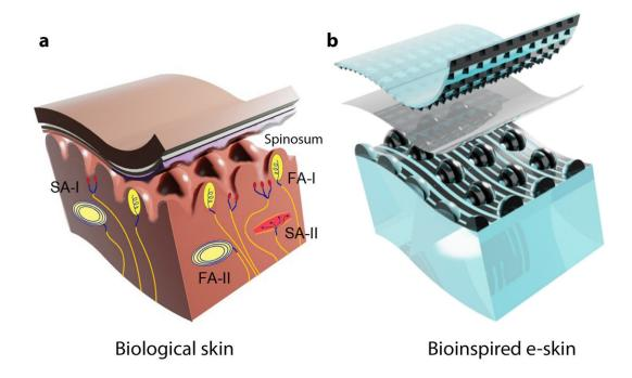
A cross-section of human skin from the fingertip depicting key sensory structures (left). This structure served as inspiration for the design of the e-skin (right). Credit: Boutry et al., *Sci. Robot.* 3, eaau6914 (2018)
