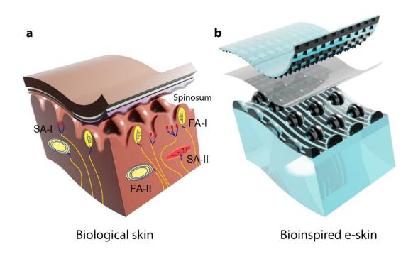
A cross-section of human skin from the fingertip depicting key sensory structures (left). This structure served as inspiration for the design of the e-skin (right). Credit: Boutry et al., *Sci. Robot.* 3, eaau6914 (2018)
