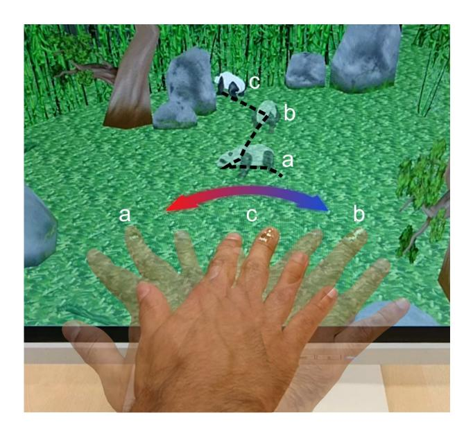
No bulky gloves, no sophisticated camera systems -- just an ultra-thin golden foil on the middle finger. That's all the Dresden researchers need to control a virtual panda with the help of the Earth's magnetic field. When the hand swipes left,
