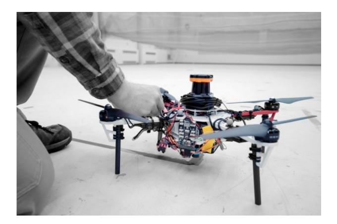
MIT researchers describe an autonomous system for a fleet of drones to collaboratively search under dense forest canopies using only onboard computation and wireless communication — no GPS required. Credit: Melanie Gonick
