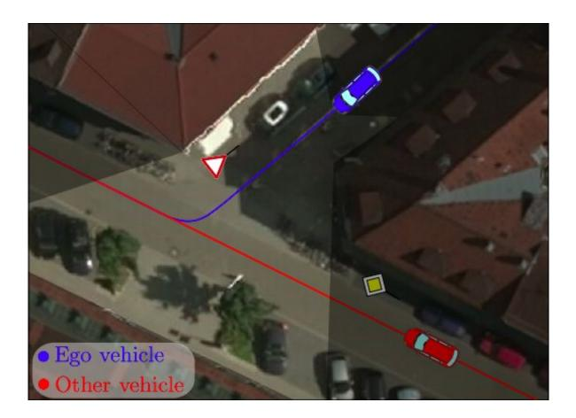
An exemplary intersection scenario highlighting a use case of the proposed approach. The ego vehicle, depicted in blue throughout this paper, proceeds to an intersection at which it has to yield to. The vehicle has limited visibility and an intersecting vehicle is approaching from the occluded region. The planner of the vehicle has to consider that there might be a vehicle approaching and adequately reduce its speed. Credit: Tas & Stiller.
