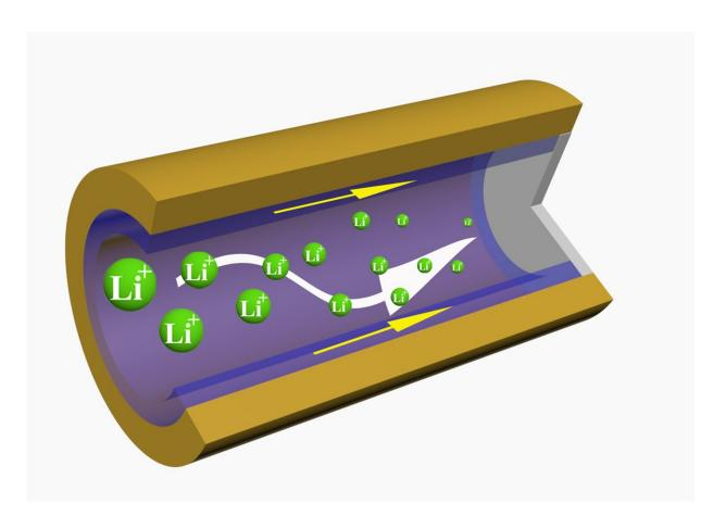
A three-dimensional cross-linked polymer sponge attaches to the metal plating of a lithium ion battery anode, allowing ion transfer and limiting deterioration. Credit: Donghai Wang, Penn State
