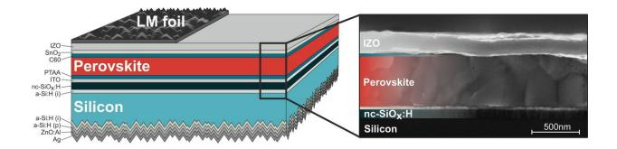
Above the perovskite layer, a structured polymer film provides better light capture. Credit: HZB
