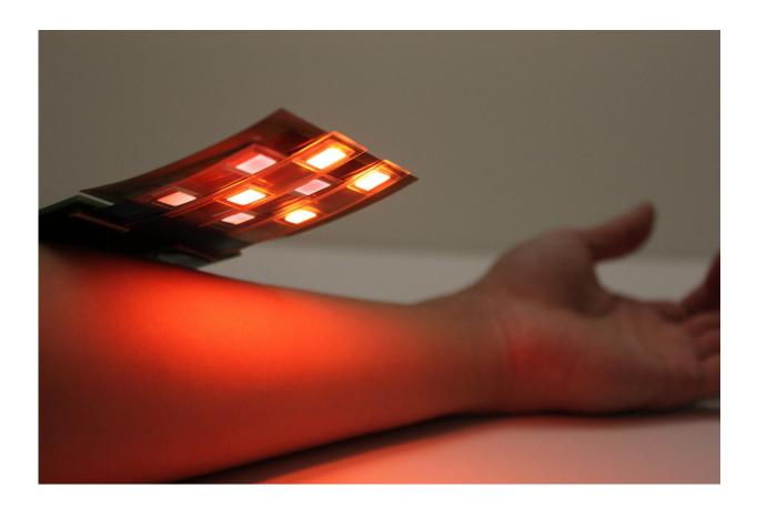
A new sensor made of an alternating array of printed light-emitting diodes and photodetectors can detect blood-oxygen levels anywhere in the body. The sensor shines red and infrared light into the skin and detects the ratio of light that is reflected back. Credit: Yasser Khan, Arias Research Group, UC Berkeley
