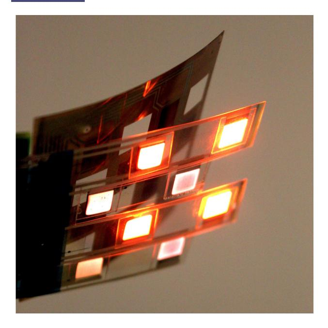
The sensor is assembled from a printed sheet of organic photo detectors (top) and organic red and infrared LEDs (bottom). Credit: Yasser Khan, Arias Research Group, UC Berkeley
