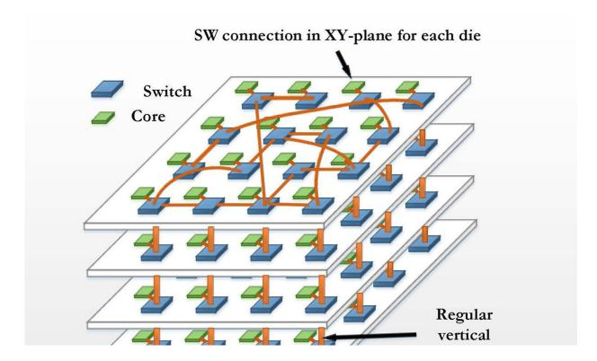
This figure shows a 3D manycore chip where the processing cores are connected through vertical links. Credit: Washington State University
