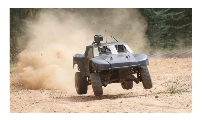
AutoRally vehicle navigating a bump on the track at high speed during testing. Credit: Drews et al.
