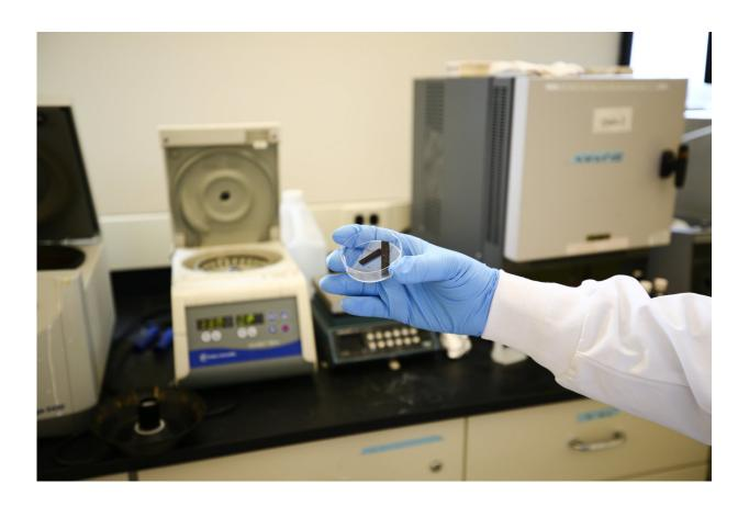
The researchers show a wafer coated in their new catalyst, which lowers the amount of electricity required to split water into hydrogen and oxygen under pH-neutral conditions. Credit: Tyler Irving/U of T Engineering
