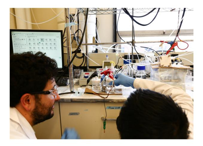
Pelayo and Dinh use their catalyst in an electrolyzer that splits water into hydrogen and oxygen. Credit: Tyler Irving/U of T Engineering
