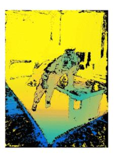
Left: Custom rig used to collect training data. Middle: An example capture flipping between the five images. Synchronization between the cameras ensures that we can calculate depth for dynamic scenes, such as this one. Right: Ground truth depth. Low confidence points, i.e., points where stereo matches are not reliable due to weak texture, are colored in black and are not used during training. Credit: Sam Ansari and Mike Milne
