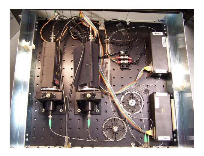
A look inside a prototype of the hardware that exchanges quantum cryptography keys. Credit: National Institute of Standards and Technology/Wikimedia
