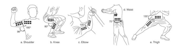
RF-Wear technology developed at Carnegie Mellon University calculates skeletal motion by analyzing radio signals reflected by RFID tags positioned on either side of each joint. Credit: Carnegie Mellon University
