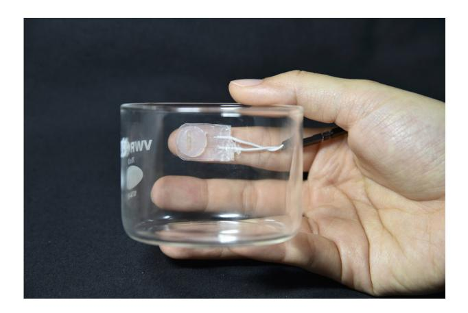
Safe, soft sensors on the top and tip of the index finger detect the movements, strain and force of the finger while performing different activities, such as flexing and extending the finger and picking up weights and boxes. Credit: Siyi Xu, Daniel M. Vogt, and Andreas W. Rousing/Harvard SEAS
