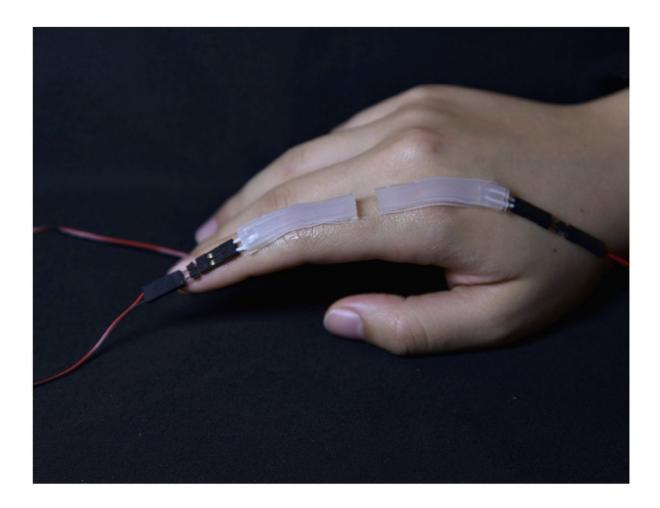
Safe, soft sensors on the top and tip of the index finger detect the movements, strain and force of the finger while performing different activities, such as flexing and extending the finger and picking up weights and boxes. (Image/video courtesy of Siyi Xu, Daniel M. Vogt, and Andreas W. Rousing/Harvard SEAS) Credit: Siyi Xu, Daniel M. Vogt, and Andreas W. Rousing/Harvard SEAS
