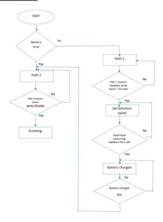
Algorithm of the functioning of Self-sustainable robot from e-scrap using renewable energy (Scrapino). Credit: Hoxha, Bula & Hajrizi.
