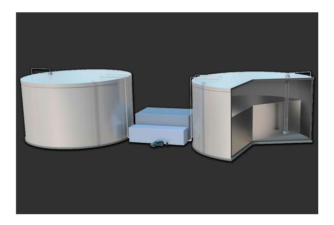
MIT researchers propose a concept for a renewable storage system, pictured here, that would store solar and wind energy in the form of white-hot liquid silicon, stored in heavily insulated tanks. Credit: Duncan MacGruer
