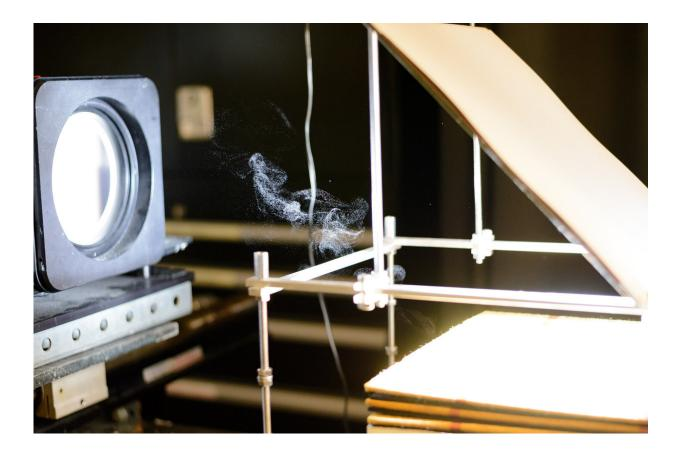
Photograph of solar-generated vapour droplets rising through a beam of simulated sunlight during a laboratory experiment with the contactless solar evaporation structure. Credit: George W. Ni
