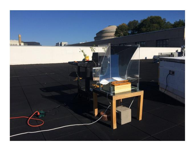
Photograph of the outdoor experiment on the MIT roof. Steam generating device is mounted over a basin of water, placed on a small table, and partially surrounded by a simple, transparent solar concentrator. Researchers measured the temperature of the steam produced over the course of the test day, October 21, 2017. Credit: researchers, Thomas Cooper *et al*.
