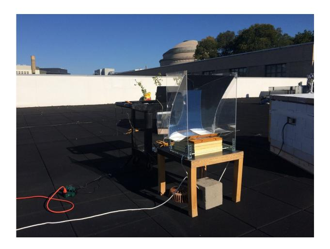
Photograph of the outdoor experiment on the MIT roof. Steam generating device is mounted over a basin of water, placed on a small table, and partially surrounded by a simple, transparent solar concentrator. Researchers measured the temperature of the steam produced over the course of the test day, October 21, 2017. Credit: researchers, Thomas Cooper *et al.*
