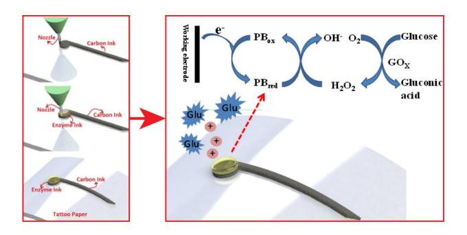
Graphic shows the 3D printed biosensor for glucose sensing, and illustrates the direct-ink-writing of electrode and enzyme ink. Credit: WSU
