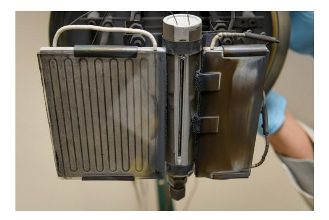
The exit slit and heater assembly of the IEC-designed and fabricated source head used to deliver doped cadmium telluride vapor to the substrate. Credit: University of Delaware
