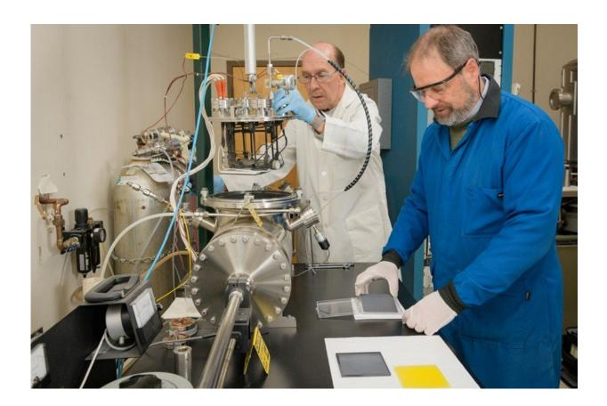
IEC researchers Wayne Buchanan (left) and Brian McCandless (right) prepare to load the vapor transport deposition system for a doped cadmium telluride film run. Buchanan is raising the source head out of the main chamber and McCandless is examining the previous film deposition (gray plate) and preparing to place the nanocrystalline film-coated glass substrate onto the graphite susceptor. Credit: University of Delaware
