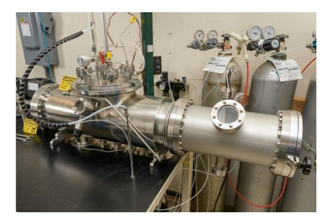
This is the vapor transport deposition system designed and built at UD's Institute of Energy Conversion to improve efficiency and lower costs of thin-film photovoltaics. Credit: University of Delaware
