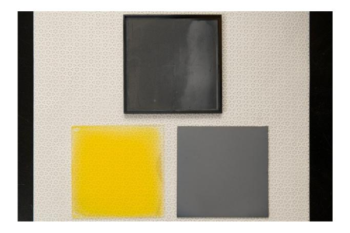
Overhead shot of the graphite susceptor (top), a nanocrystalline film-coated glass substrate (yellow) and a completed stack with the doped cadmium telluride film (gray). Credit: University of Delaware
