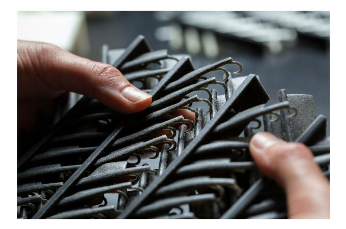
Researchers 3D-printed structures that mimic the feathers' vanes, barbs and barbules to better understand their properties--for example, how the underside of a feather can capture air for lift, while the top of the feather can block air out when gravity needs to take over. Credit: University of California San Diego
