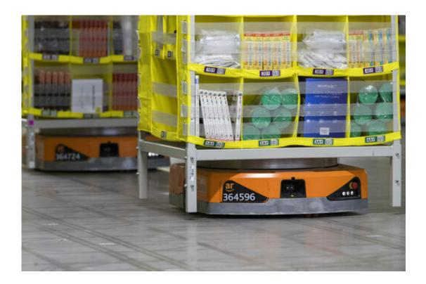
In this Dec. 5, 2018, photo pods full of merchandise are moved around the floor by robotic drives, named Amazon robots, at the Amazon fulfillment center on Staten Island borough of New York. Robots aren't replacing everyone, but a quarter of U.S. jobs will be severely disrupted as artificial intelligence accelerates the automation of today's work, according to a new Brookings Institution report published Thursday, Jan. 24, 2019. (AP Photo/Mary Altaffer)
