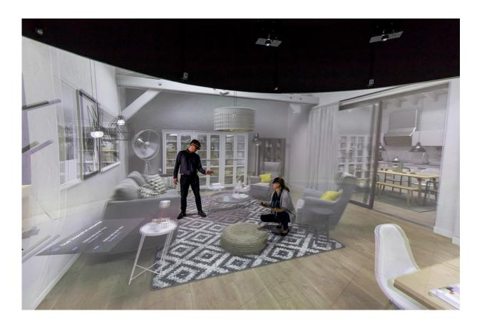
The stereoscopic projection system makes it possible to perceive virtual worlds in the Elbedome in three dimensions. Holographic representation gives users the sense of being in the midst of the projected images. Credit: Fraunhofer-Gesellschaft
