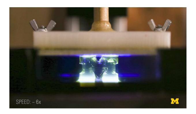
Rather than building up plastic filaments layer by layer, a new approach to 3-D printing lifts complex shapes from a vat of liquid at up to 100 times faster than conventional 3-D printing processes, University of Michigan researchers have shown.
