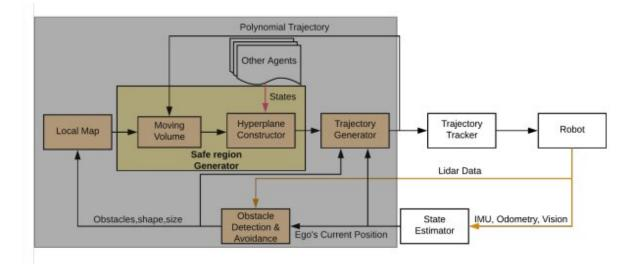
The system overview of an individual agent. The orange arrows represent raw data,red represent data from external sources and black represent processed data and flow side. The focus of this work is the shaded portion. Credit: Govind Aadithya R et al.
