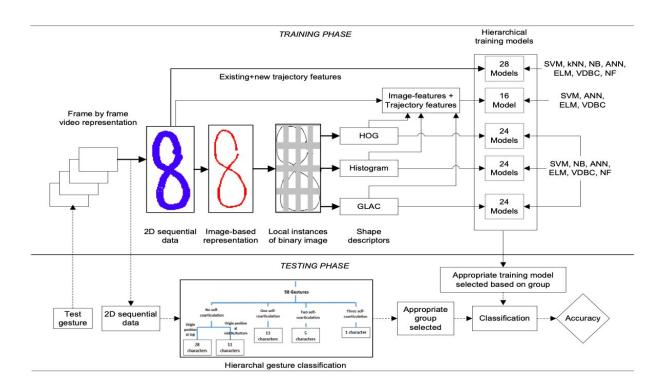
Block representation of training (hard and dotted lines) and testing (dashed lines) phase of the proposed system. Credit: S. Misra & R. H. Laskar.
