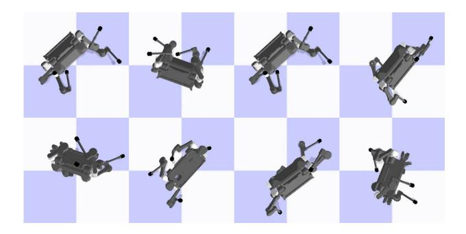
Different fall configurations of the ANYmal robot. Credit: Hwangbo et al., Sci. Robot. 4, eaau5872 (2019)
