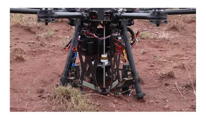
How to dig a hole with two drone and a parachute. That's a headline painfully hard to skip over and we did not. *IEEE Spectrum* is reporting on the portable digging system that is proving up to the many-faceted task: keeping a useful distance, locating a spot that is diggable, landing, then verifying that the spot really is diggable, proceeding to dig a hole and install a sensor, and fly off.
