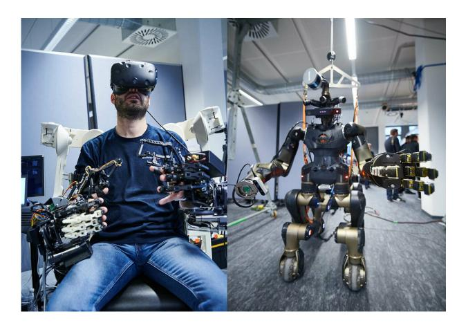
Tele-operated robot Centauro can fulfil tasks such as climbing stairs, navigating obstacles and using power tools. Credit: Centauro
