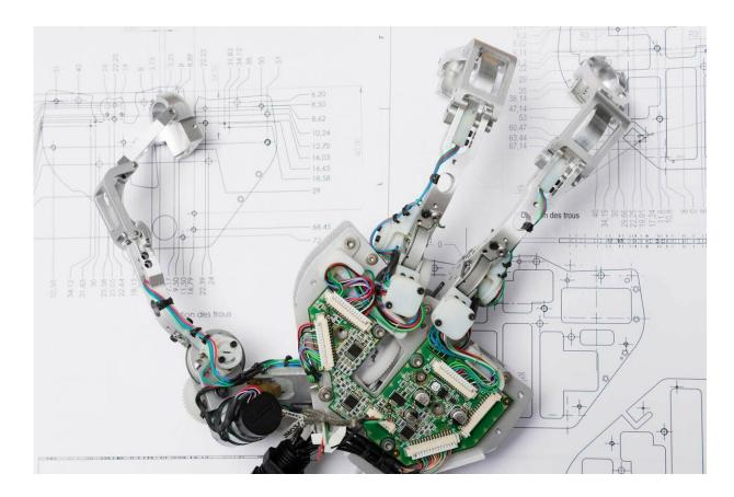
The three-fingered hand exoskeleton developed by CEA captures the operator's movements to control the slave robot hand. Credit: CEA / Stroppa
