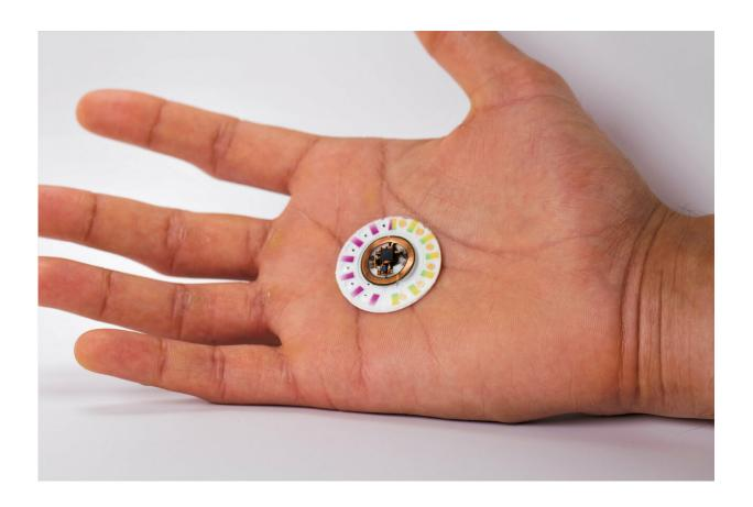
Picture of a microfluidic device designed to mount on the skin and to collect and analyze microliter volumes of sweat. The system includes combined capabilities in electrical and color-based measurements of the rate and loss of sweat, as well as the concentrations of glucose, lactate and chloride and the pH level. Credit: J. Rogers, Northwestern University
