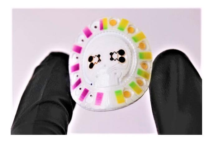
Picture of a flexible microfluidic module for collecting sweat and measuring the rate of sweat release, the total loss of sweat, the concentration of chloride and the pH level. Credit: J. Rogers, Northwestern University
