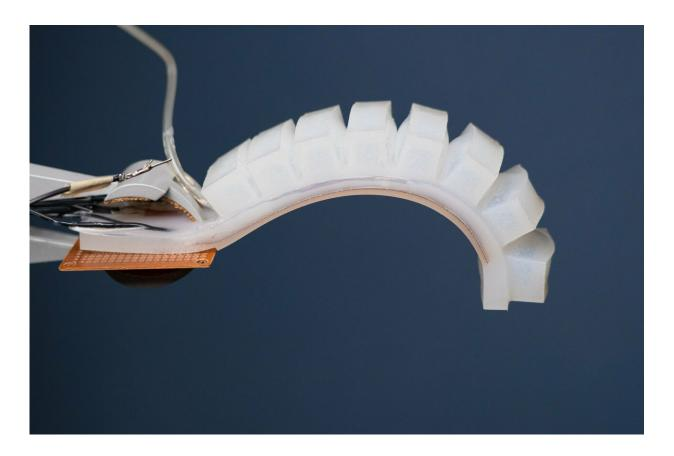
The soft robotic finger provides haptic and movement information to the system. Credit: University of California San Diego
