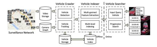
The architecture of the progressive vehicle search system. Credit: Liu et al.
