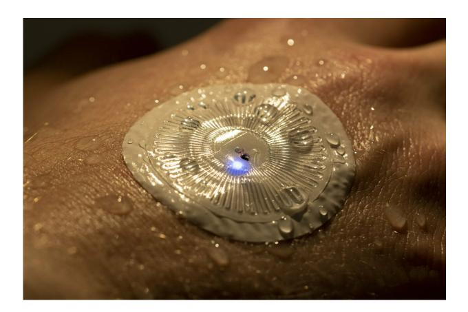
An electronics-enabled epidermal microfluidic system mounted on the back of the hand transmits skin temperature to an external smartphone via NFC and displays notifications to the user via an on-board LED. Credit: John Rogers Research Group
